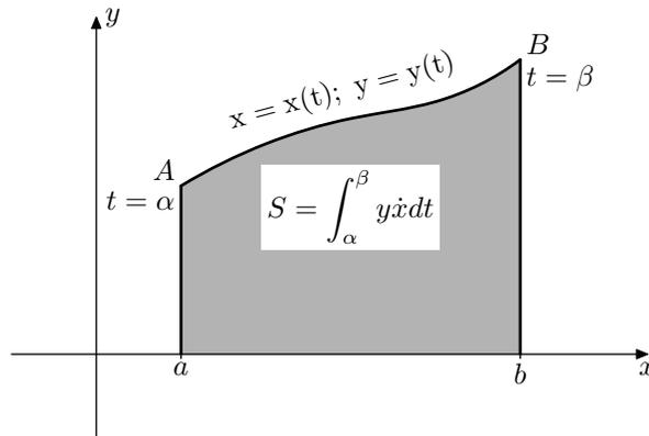
Figure 5.7. The area under the graph of the curve  $x = x(t)$ ,  $y = y(t)$
