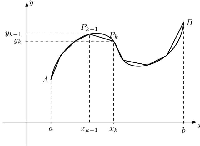
Figure 5.15. The approximation of the curve by a series of straight lines
