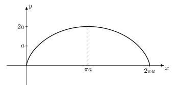
Figure 5.16. The arc of cycloid for  $t \in [0; 2\pi]$
