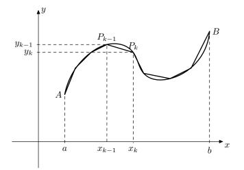
Figure 5.15. The approximation of the curve by a series of straight lines
